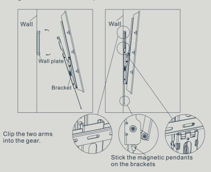
(1)Press the brackets after you put them on the wall plate, then they would be locked with wall plate.
