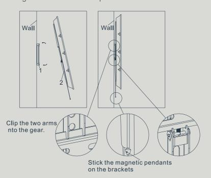
(1)Press the brackets after you put them on the wall plate, then they would be locked with wall plate.
